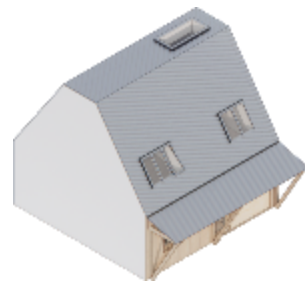
Roof eaves - big (1,5 m)
