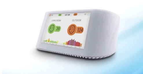
Figure 5: AirVisual Pro, a device for continuously measuring comfort parameters
