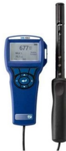
Figure 3: IAQ-Calc 7545 portable detector for measuring CO 2 , T, RH and CO
